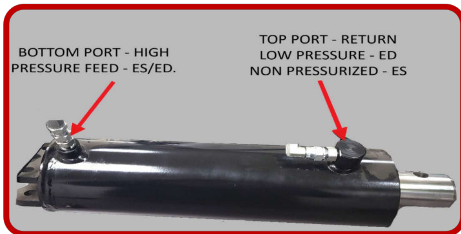
FIGURE 9: CYLINDER PORTS
