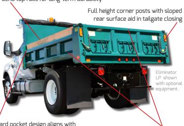
Board pocket design aligns with cabshield and allows the use of tapered side boards to increase capacity when hauling lighter loads such as brush, firewood, and mulch
