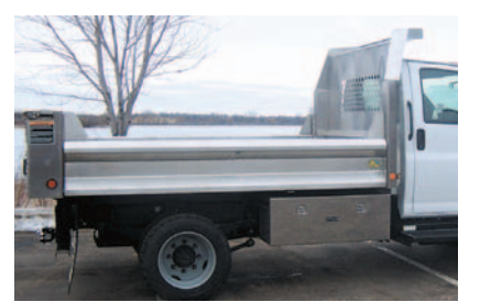
Body shown with standard sides and tall cab shield
