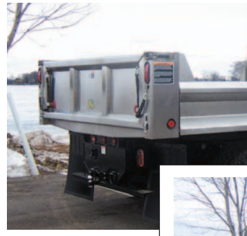
Stainless steel body features a vertical tailgate
