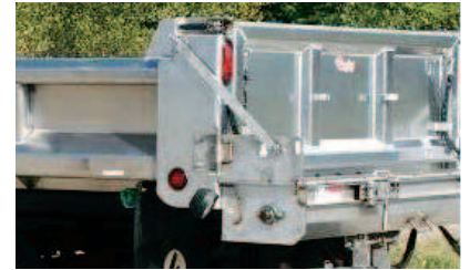
Stainless steel EZ-LATCH™ upper tailgate mechanism
