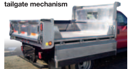
Aluminum fold-down sides provide lightweight operations.
