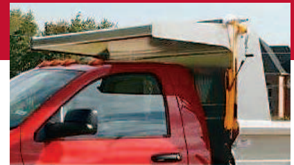
Lightweight aluminum 3/4 cab shield
