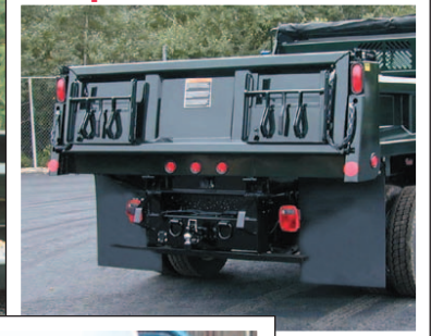
Optional coal chutes installed
